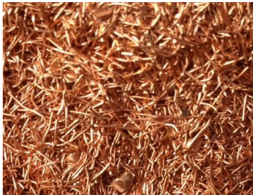
Separated flexible cable copper 2 up to 20mm. Position 3
